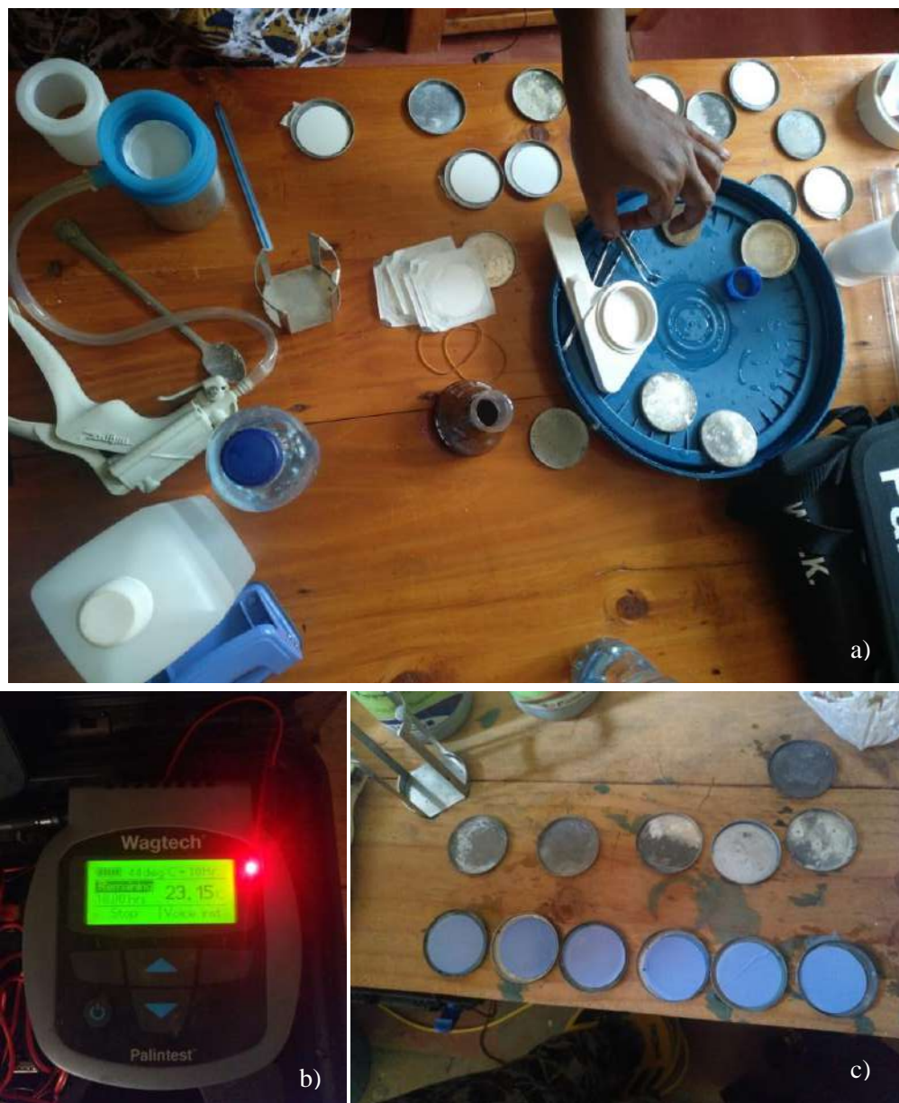
Figure 10: Faecal coliform determination: filtration equipment (a), setting the incubator (b) and end result with no observed colonies in the plates (c).
