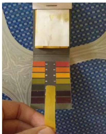
Figure 9: Turbidity test performed in the sample from the Rope Pump (left); pH strip showing the range for the water collected in the dispensary.
