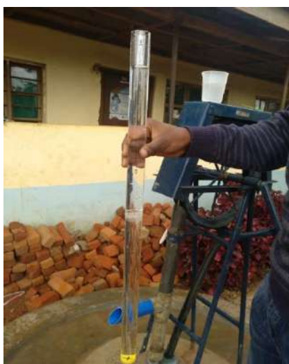
Figure 9: Turbidity test performed in the sample from the Rope Pump (left); pH strip showing the range for the water collected in the dispensary.
